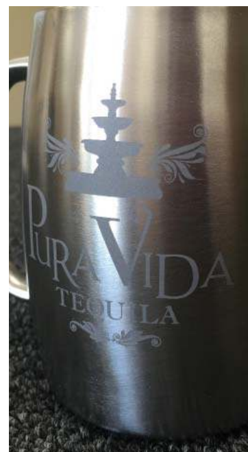
(above) Careful masking is imperative to ensuring clean lines when sandcarving or blasting metal items, and creates a template for any painting or color-filling to be done later.
